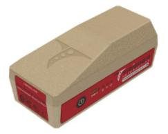
**Switch Module:** Will be used to either hide or expose flags. This also starts a time when exposed and records until it is hit. Then it sends the data back to the central module for the user to see.
