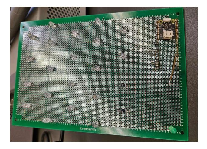
Raspberry Pi Pico: used to control and receive input from sensors.
